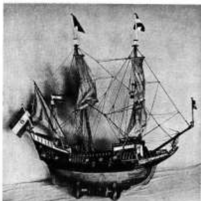
A scale model of Tasman's flagship, Zeekam . Square-rigged with a high poop, she was approximately 100 feet long and could be compared in size with the Mayflower which took the Pilgrim Fathers to America.
